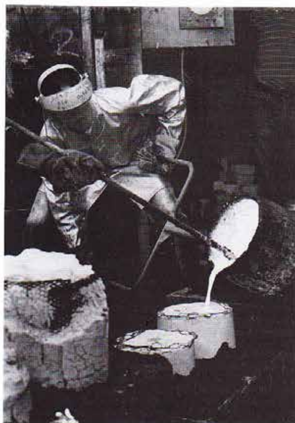
7. Casting bronze using the conventional process: the sculpture foundry of the Pennsylvania State University.
