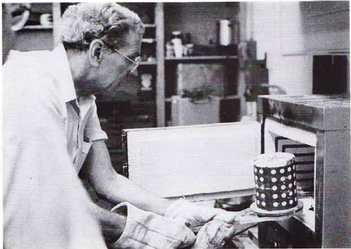
5. Norman Willis, curator of medals in Canada's public archives, withdraws the flask from the kiln in preparation for the bronze pour.
