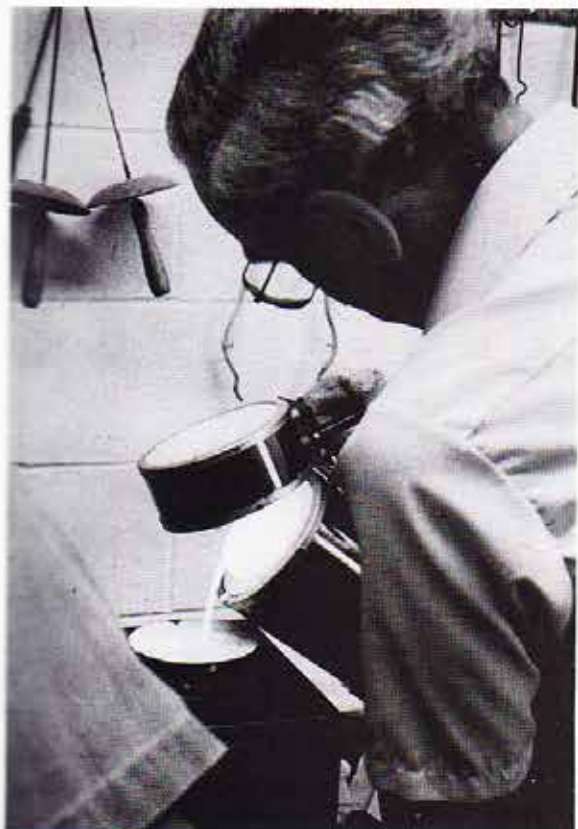
6. Norman Willis pours a cluster of medals, using a small electric portable furnace not unlike a coffee-pot.
